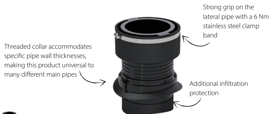
FA150B: Lateral Pipe Multibush Configuration
